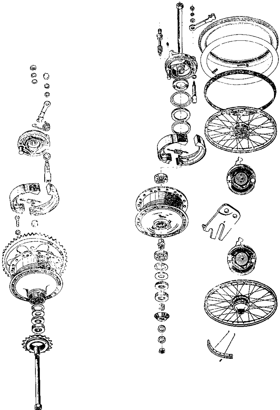
Fig. 26 Exploded view of front and rear wheel.
