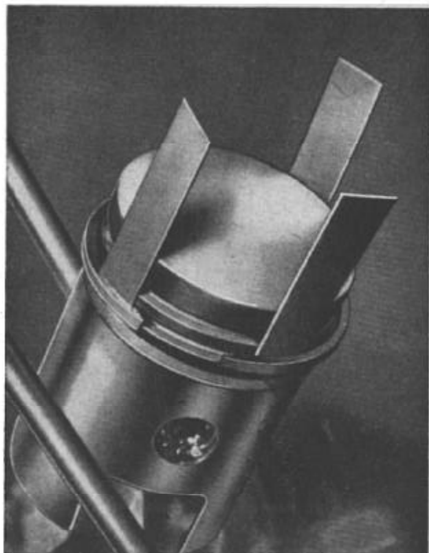
26. Replacing the piston rings.
